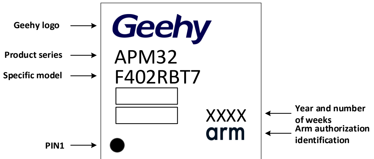
Figure 18 LQFP64 - 64 Pins, 10 x 10mm Package Identification
