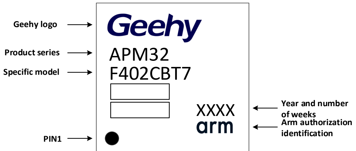
Figure 21 LQFP48 -48 Pins, 7x7mm Identification
