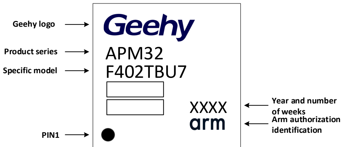
Figure 27 LQFN36-36 Pin 6x6mm Identification
